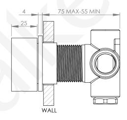
Ensure water lines are completely flushed prior to connecting the mixer.
