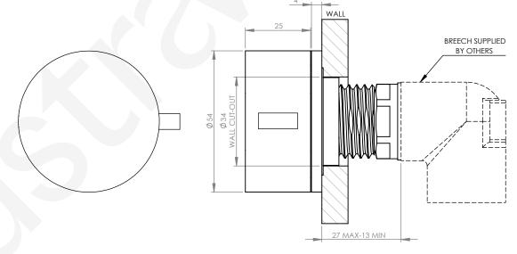
IMPORTANT: Front face of inwall body to finished wall face must be minimum 13mm to maximum 27mm
