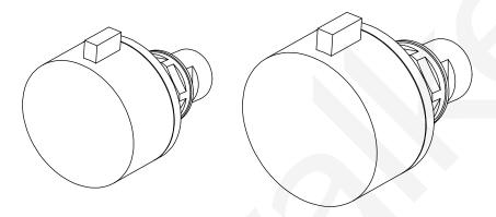
Install the wall breech (not supplied) to a secure nogging at the correct depth as shown in the drawing below. Ensure the breech is square and parallel between the wall studs.
