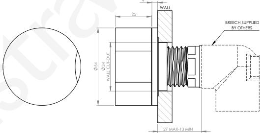
IMPORTANT: Front face of inwall body to finished wall face must be minimum 13mm to maximum 27mm
