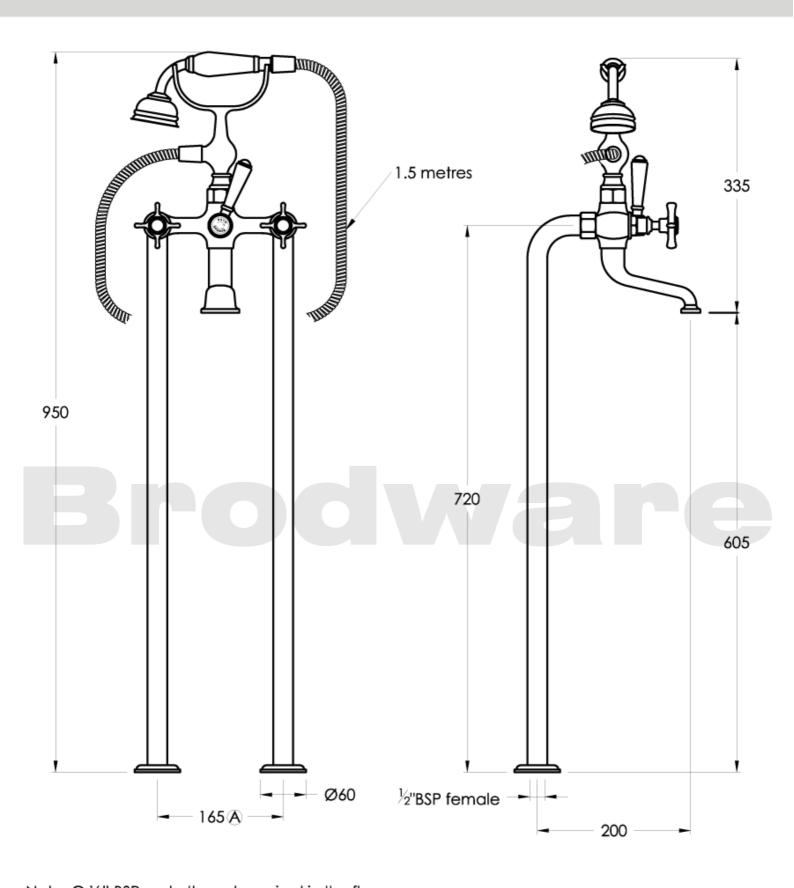
Note: G ½" BSP male thread required in the floor (A) Fixed centre; outlets must have 165mm centres
