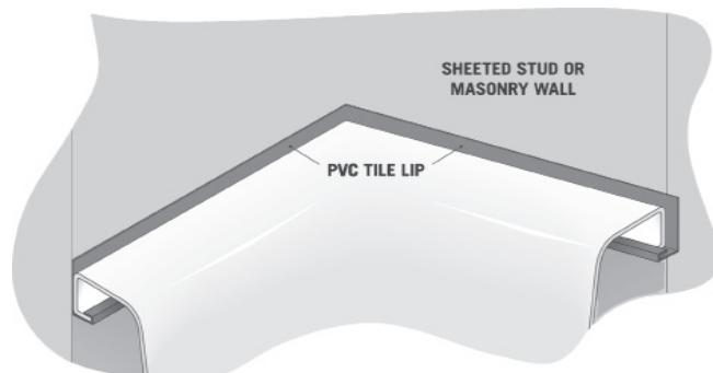
When the bath is installed, the minimum distance from the outside edge of the flange to the finished edge of the tiles shall be 10mm. The exposed area of the flange shall have continuous fall to the inside of the bath.
