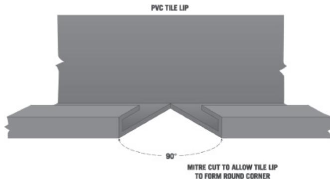
This clip on material should be cut to the required lengths, mitred at the corners, and the area where the flashing material and the rim of the bath meet, should be filled with a mould resistant Sanitary Grade sealant.
