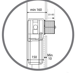
Cavity & wall thickness to be a minimum of 10mm
