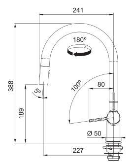
**PLEASE NOTE:** Large and heavy taps should ideally be mounted directly through the solid benchtop or fully supported from underneath. For all other swivel taps, we recommend the use of the Franke Tap Support Arm to provide additional support. Please ensure all Franke tapware is installed at a pressure of no greater than 500 kPa in accordance with AS/NZS3500 and insist that your plumber flushes all of the water supply lines before installing tapware. Failure to do so may void warranty.
